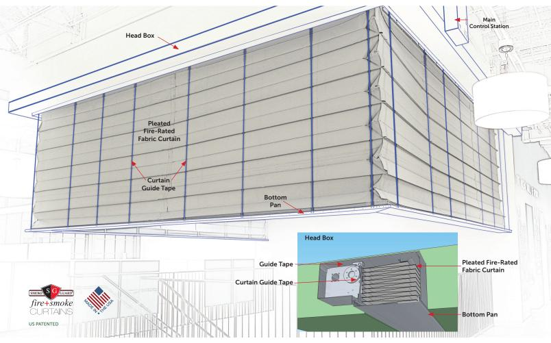
**System Operation.** The system is deployed upon a signal from the local smoke detection system or a smoke control panel. System requires 120-240 volt power. The unit is also equipped with a 24 volt DC battery back-up system that maintains the electronic controls. When required the system can be connected to building standby power. The controls include a universal power supply that supports either 120 or 240 volt operation.
